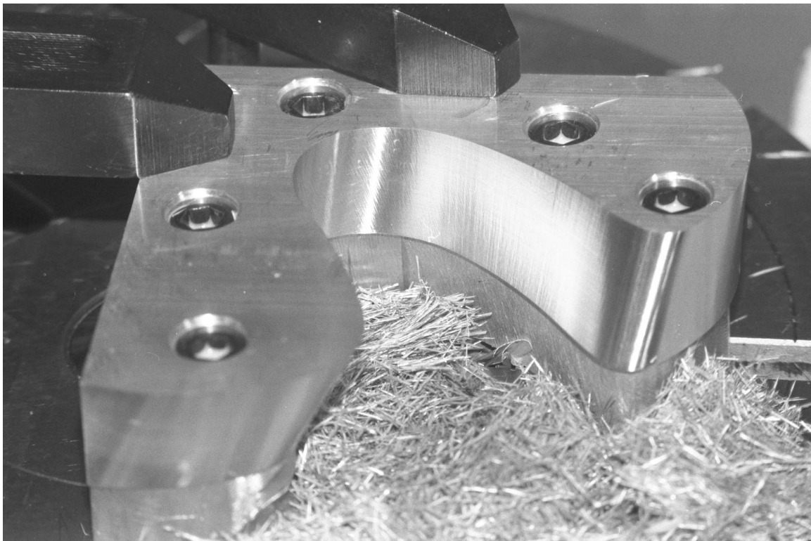
Fig. 15. Photographs of the machined part and 25.4 mm diameter flat end-mill cutter.
